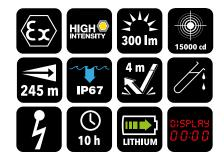
ATEX: II 1G Ex ia op is IIC T4 Ga II 1D Ex ia op is IIIC T85°C Da GAS ZONE 0 | 1 | 2 DUST ZONE 20 | 21 | 22 Step Lighting System
