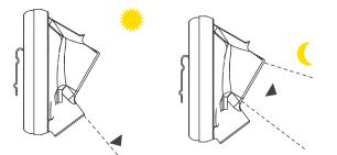
The intensity and the direction of the light beam are managed automatically by means of an enviroment light sensor: it avoids optical harm among the users and saves battery duration.
