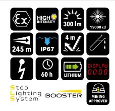
ATEX: II 1G Ex ia op is IIC T4 Ga II 1D Ex ia op is IIIC T135°C Da I M1 Ex ia op is I Ma
