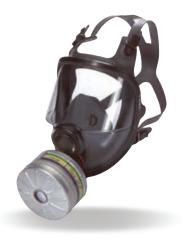
For gases and vapours: NPF 2,000 - APF 20\* For particulates with P3: NPF 2,000 - APF 40 For gases with P3: NPF 2,000 - APF 20\* For Class 1 gas filters : 10 or up to 1,000 ppm (whichever is the lower) For Class 2 gas filters: 10 up to 5,000 ppm
