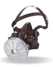
For gases and vapours: NPF 50 - APF 10\* For particulates with P3: NPF 50 - APF 20 For gases with P3: NPF 50 - APF 10\* \* For Class 1 gas filters: 10 or up to 1,000 ppm(whichever is the lower) \* For Class 2 gas filters: 10 or up to 5,000 ppm
