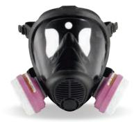
For gases and vapours: NPF 2,000 - APF 20\* For particulates with P3: NPF 2,000 - APF 40 For gases with P3: NPF 2,000 - APF 20\* For Class 1 gas filters: 10 or up to 1,000 ppm (whichever is the lower) For Class 2 gas filters: 10 up to 5,000 ppm (whichever is the lower)
