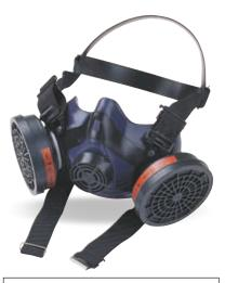
For gases and vapours: NPF 50 - APF 10\* For particulates with P3: NPF 50 - APF 20 For gases with P3: NPF 50 - APF 10\* \* For Class 1 gas filters: 10 or up to 1,000 ppm (whichever is the lower) \* For Class 2 gas filters: 10 or up to 5,000 ppm (whichever is the lower)
