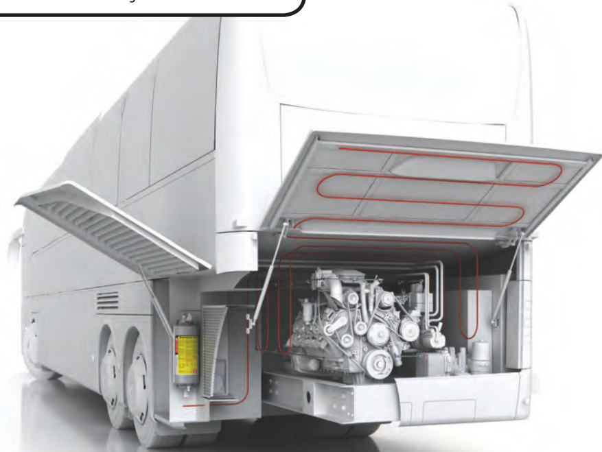
*Red tubing for visualization only. System is installed with black tubing
