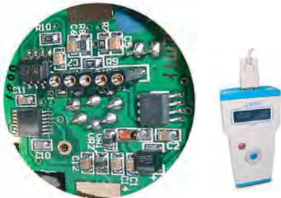
DIMES valves contain a micro chip that permits calibration of the system to the cylinder of valves. A calibration unit is required
